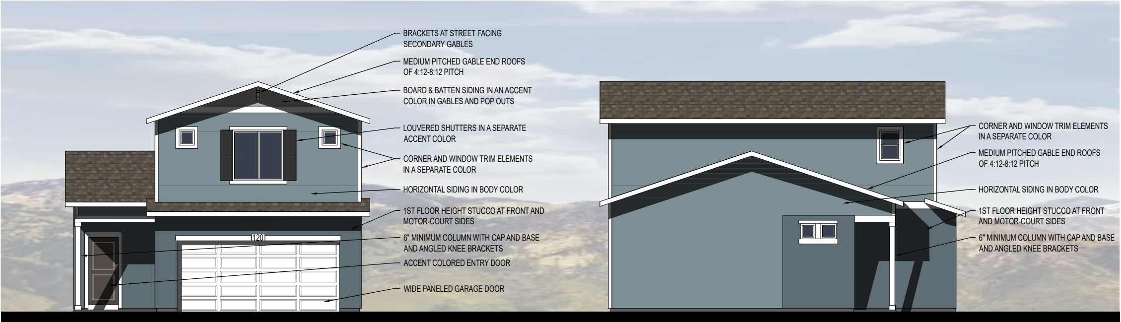
1 Typical Front Elevation - Motorcourt Interior Location Plan 120 shown
